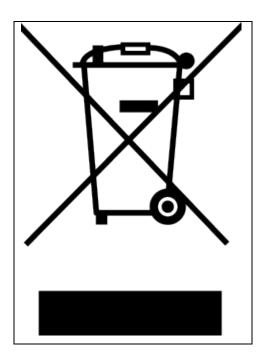
The horizontal bar underneath the crossed-out wheelie bin indicates that the equipment has been manufactured after the Directive came into force in 2005. The wheelie bin symbol is added to the type designation label of the product since 2017. The figure below shows an example.
