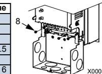
8. Install conduit/gland box and tighten the cable clamps.
