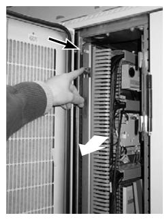
To push the control unit back into the cubicle:
