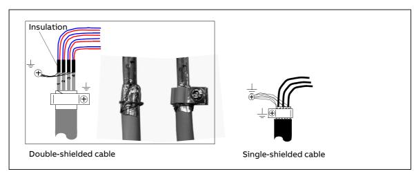
When the outer surface of the shield is covered with non-conductive material:
