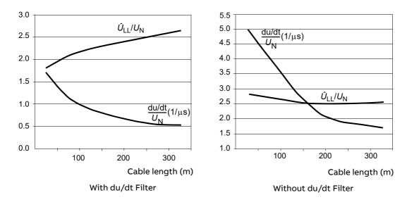
**Note 10:** Sine filters protect the motor insulation system. Therefore, du/dt filter can be replaced with a sine filter. The peak phase-to-phase voltage with the sine filter is approximately  $1.5 \times U_N$ .
