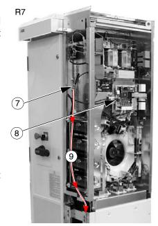
10. Remove screws fastening the drive module trolley to the pedestal.
