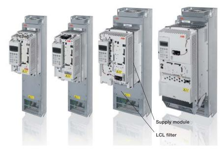
The regenerative IGBT supply unit consists of a supply module and an LCL filter. The filter suppresses the AC voltage distortion and current harmonics.
