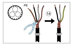
15. Connect the cable as the motor cable in step 8. Ground the shield 360 degrees (15a). Connect the twisted shield to the grounding terminal (15b) and the conductors to the R+ and R- terminals (15c) and tighten to the torque given below the figure.
