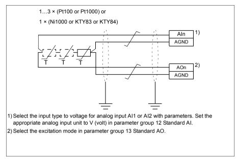
**WARNING!** As the inputs pictured above are not insulated according to IEC 60664, the connection of the motor temperature sensor requires double or reinforced insulation between motor live parts and the sensor. If the assembly does not fulfill the requirement, the I/O board terminals must be protected against contact and must not be connected to other equipment or the temperature sensor must be isolated from the I/O terminals.
