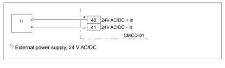
**WARNING!** Do not connect the +24 V AC cable to the control board ground when the control board is powered using an external 24 V AC supply.
