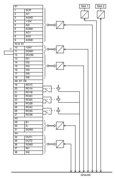
\*) Jumper installed at factory
