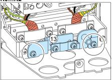
14. Repeat steps 5...7 for the brake resistor cable. Cut off one phase conductor.
