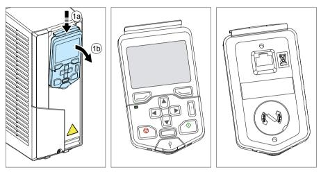
To reinstall the control panel, put the bottom of the container in position (1a), press the retaining clip at the top (1b) and push the control panel in at the top edge (1c).
