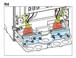
17. Put the (so far) unused rubber grommets to the holes in the lead-through plate, unless you will continue with installing the control cables.
