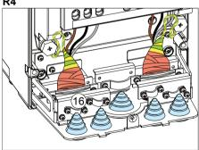
18. Secure the cables outside the unit mechanically.
