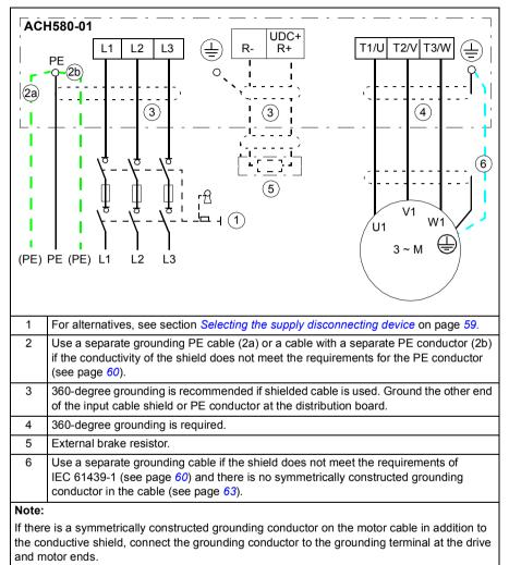
Do not use an asymmetrically constructed motor cable for motors above 30 kW (see page 60). Connecting its fourth conductor at the motor end increases bearing currents and causes extra wear.
