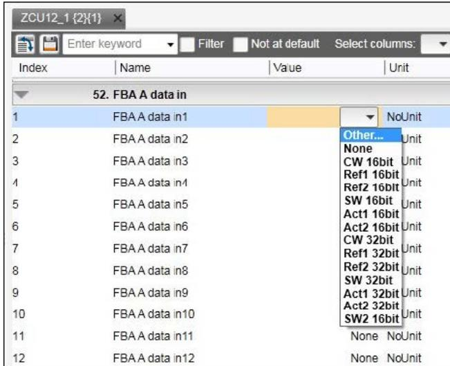
The screenshot shows a window titled "ZCU12\_1 {2}{1}" with a search bar and a table of parameters. The table has columns for Index, Name, Value, and Unit. A dropdown menu is open over the "Value" column for the first row, showing options like "None", "CW 16bit", "Ref1 16bit", etc.
