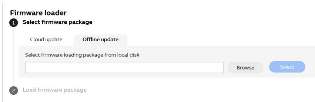
**Note:** If you try to load a corrupted or invalid loading package file, the application displays an error message.
