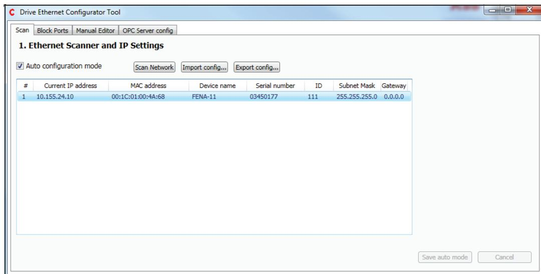
Drive Composer scans all the COM ports and Ethernet ports to find drives. If problems arise, see *Ethernet tool network for ACS880 drives application guide* (3AUA0000125635 [English]).
