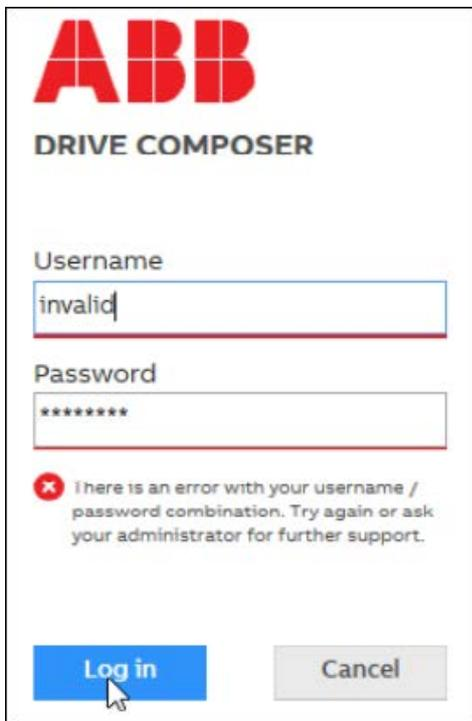
**Note:** Login is successful only when the credentials of drive match with that of RADIUS server. If the credentials are not matching, you may have to shut down the RADIUS server and login to the drive using offline credentials (i.e. service user access level). For default offline credentials, contact your local ABB representative.
