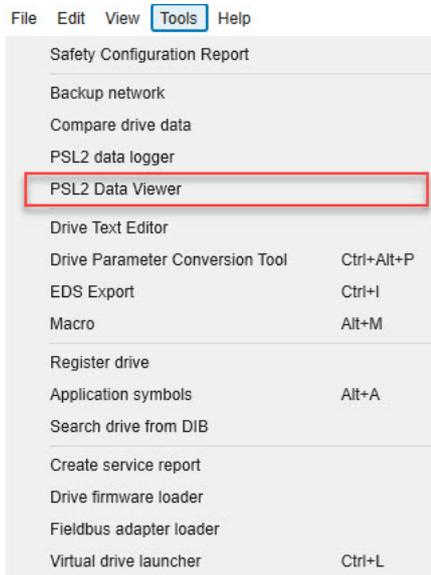
2. PSL2 Data Viewer screen with PSL2 plotting tools appears. The plotting area is empty by default. See [PSL2 Data Viewer instructions](#) below to open and save the plot.
