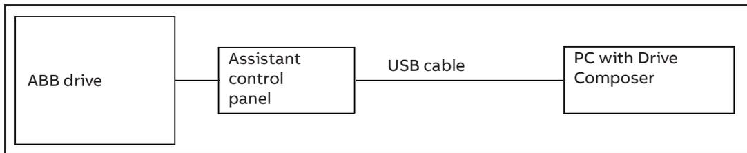
The following text appears on the Assistant control panel screen: “USB **connected**”.
