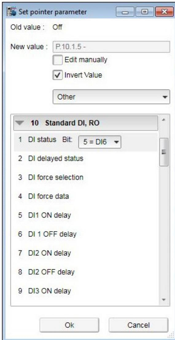
The inverted bit pointer value is shown with the minus sign at the end of the parameter.
