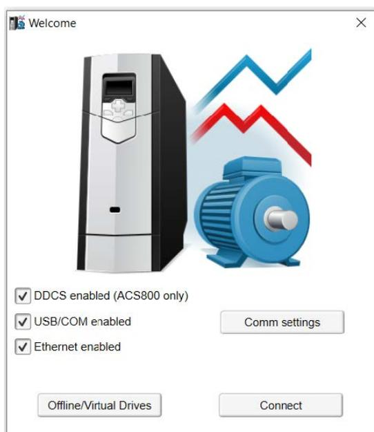
3. Click **Connect** to connect to the drive or click **Offline/Virtual Drives** to connect an offline or virtual drive. For more information, see [Virtual drives Quick installation and start-up guide \(3AXD50000422128 \[English\]\)](#) .
