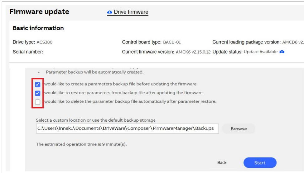
**Note:** In ACS380, for successful parameters back up and restore, the drive needs to be in local control mode. Hence, during a firmware update, if the drive is in remote control mode, the tool automatically changes it to local control mode. After the firmware update, the control mode is restored to its original mode.
