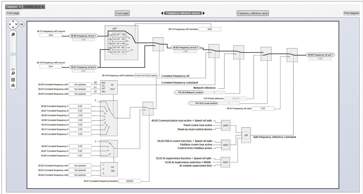
To navigate back to the top level of a Control Diagram, click the **Diagrams top** icon. To navigate through the reference chain, click the buttons circled in the figure above.
