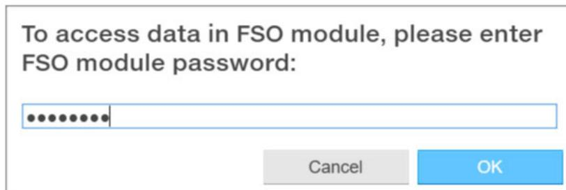
**Note:** You can change password by clicking Change password (see figure [FSO configuration: Parameter view](#)). Make sure the drive is not modulating. The password must contain 4...8 digits. Do not forget the new password; otherwise you have to do a factory reset to the FSO which clears the configuration and resets the parameters to the factory defaults.
