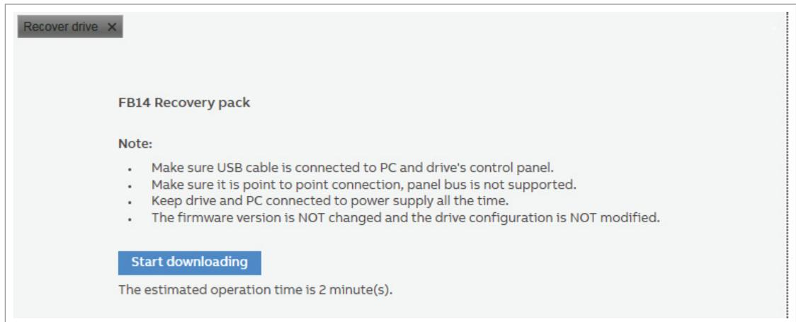
**Note:** If downloading the Recovery pack failed, follow instructions in [FB14 Recovery and Service pack failure](#).
