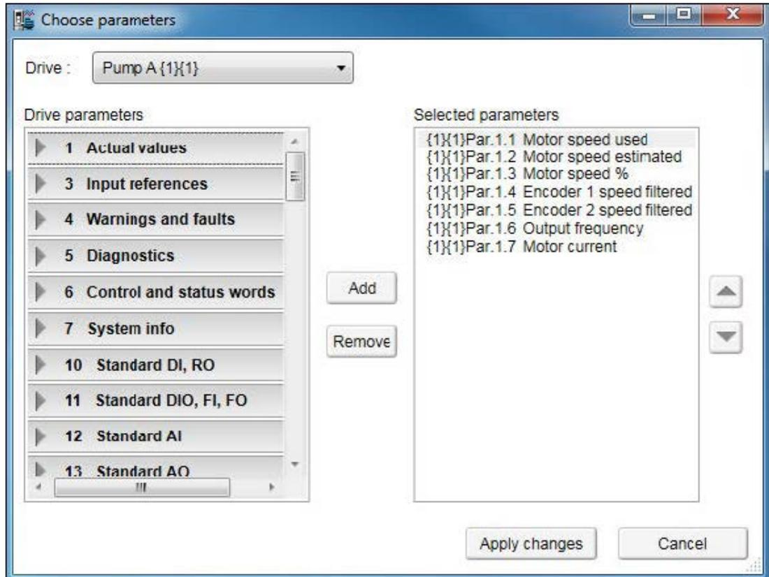
**Note:** The maximum number of signals that a logger can record at one time depends on the drive. Add button is disabled when maximum number of parameters are reached.
