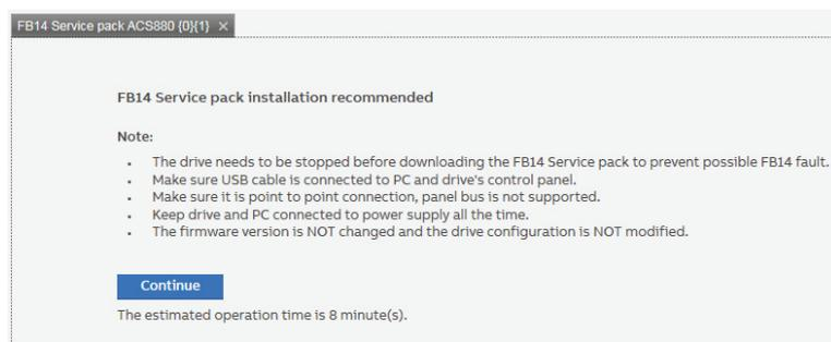
3. Before installing the Service pack, Drive Composer creates a parameter backup. Check **Parameter backup**.
