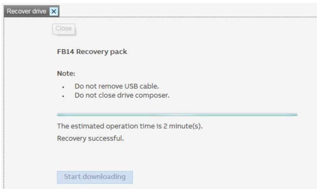
The drive may be functional now, but the fault root cause still exists in the drive. Proceed with installing [FB14 Service pack](#), to completely prevent the FB14 fault.
