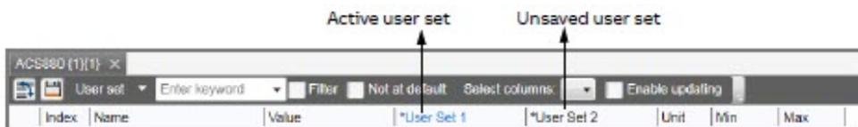
The unsaved user set is highlighted with \* symbol in the header row of the parameter window.
