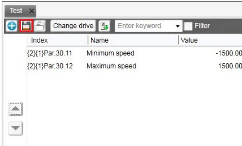
Drive Composer saves to file the values in the **Offline value** column. If the **Offline value** column was empty, then values in the **Values** column is saved.
