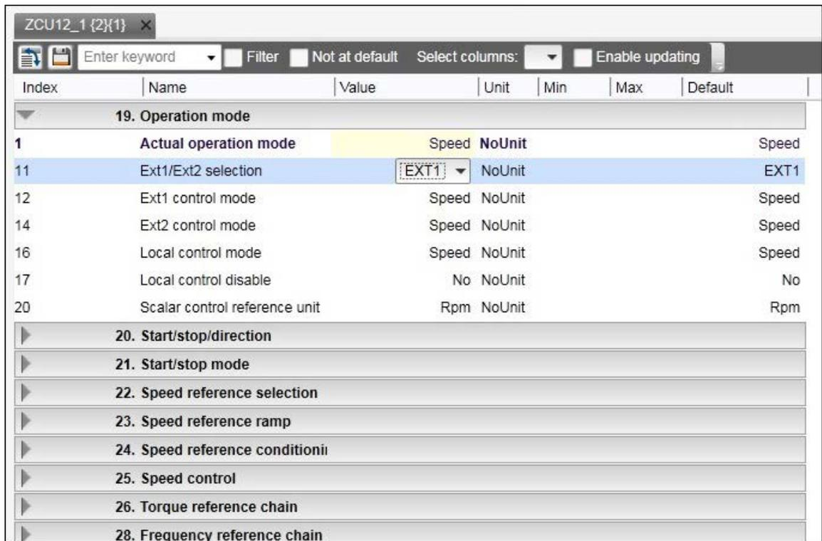
Parameters or signals can be sent to the monitor window by right-clicking them and selecting **Send to monitor**. Parameters can be copied to a custom parameter window by right-clicking them and selecting **Copy**. In addition, you can drag and drop parameters to a custom parameter window.
