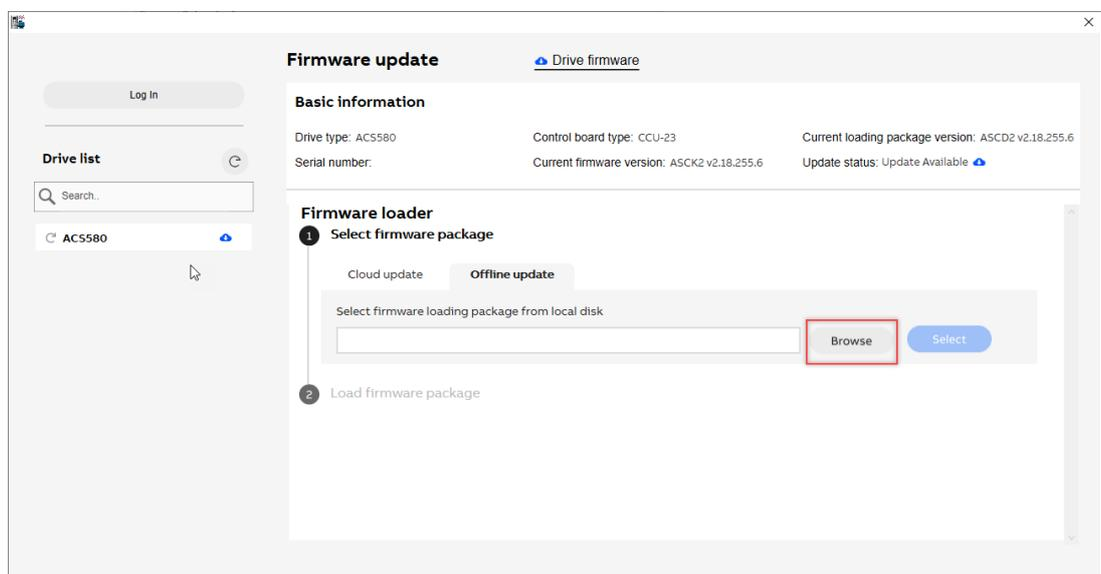
**Note:** If you try to load a corrupted or invalid loading package file, the application displays an error message.
