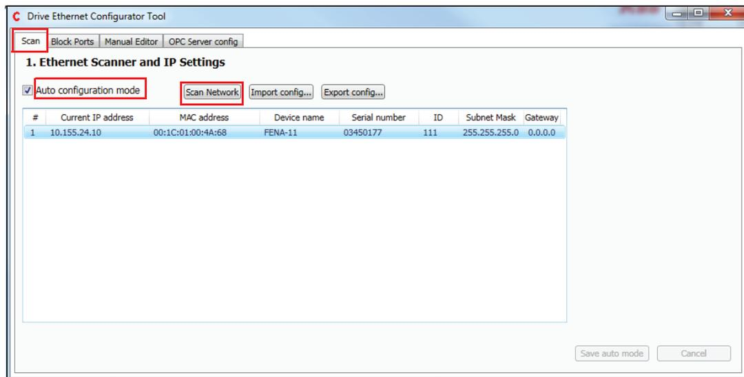
Drive Composer scans all the COM ports and Ethernet ports to find drives. For more information, see *Ethernet tool network for ACS880 drives application guide* (3AUA0000125635 [English]).
