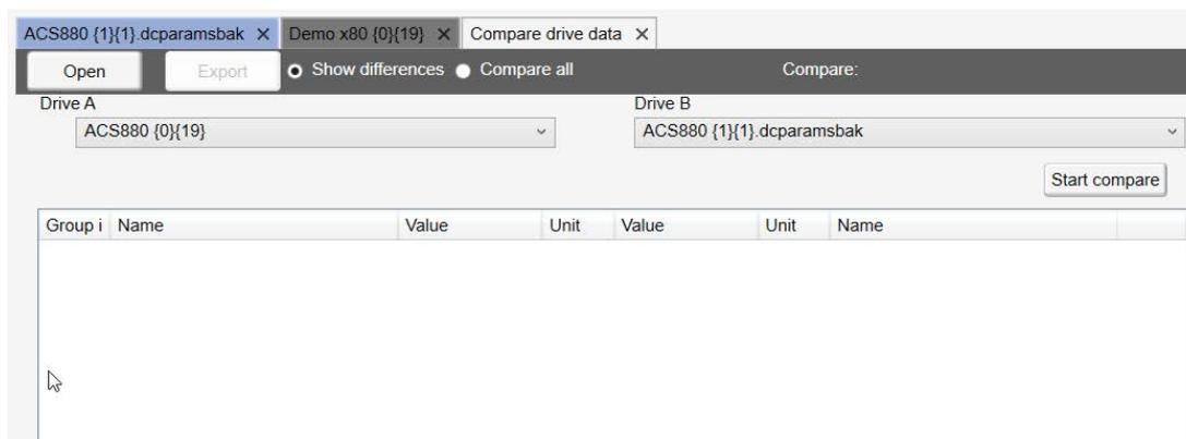
2. In a PC tool network, select drives from **Drive A** and **Drive B** drop-down menus.
