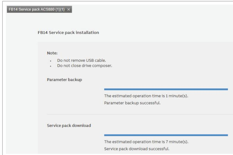
6. After installation is complete, Drive Composer sends the Service pack update event to ABB server. Later this information is maintained in the Drives Installed Base. Click **Next**.
