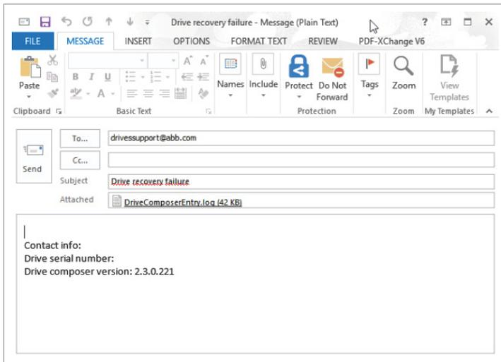
**Note:** Drive ID is filled only when the Service pack installation fails. Drive Composer attaches the log file to the mail. But you can also attach the backup file.
