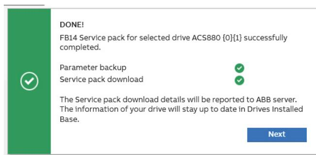
7. A thank you message appears to acknowledge the Service pack installation. You can continue using the drive with the parameter backup saved in your PC. To access the saved location, click on the link **Open file location**.
