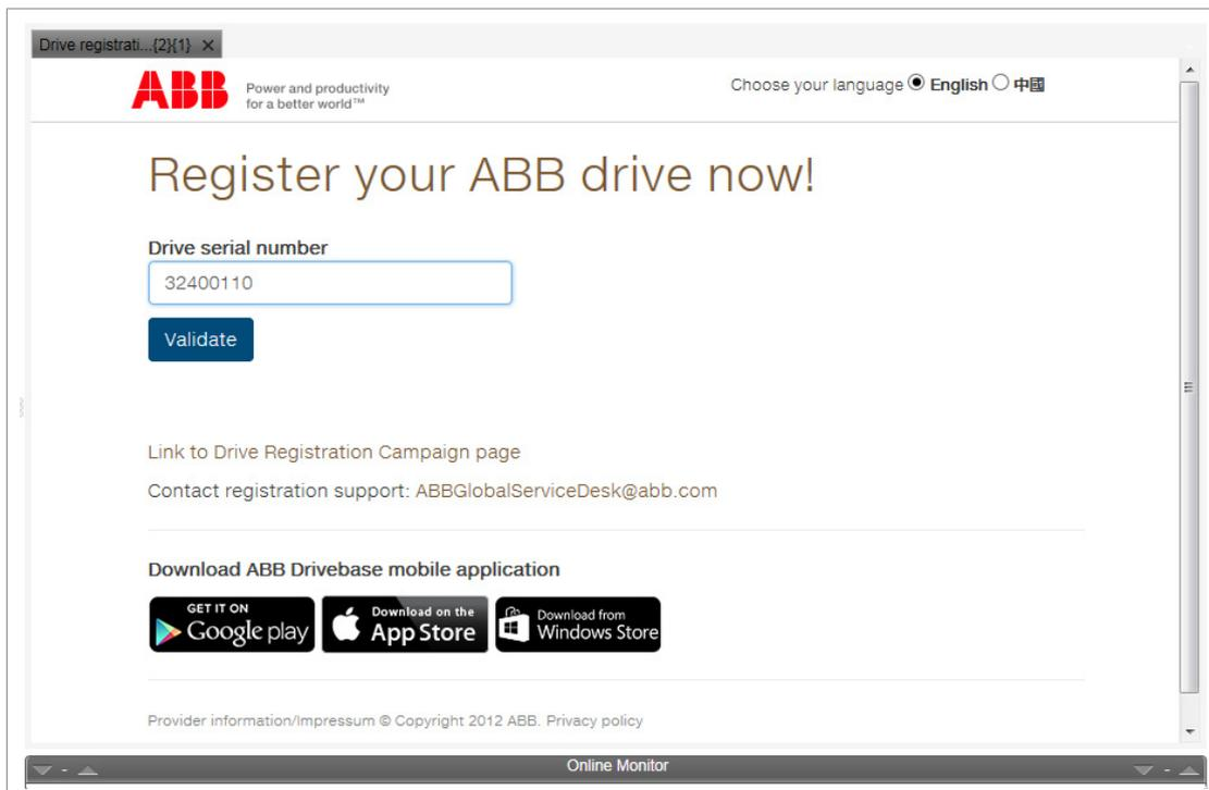
Drive Composer connects to Drive Installed Base portal (external website) and validates the serial number with an associated type code. If the number is valid, the drive type code is automatically filled. For example, PCB, CT BOARD.
