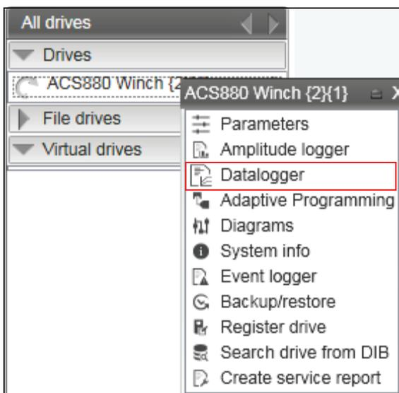
The data collecting can be stopped with a specific stop command or automatically when a triggering condition is true in the drive. After data collection stops you can read and study the data in Drive Composer pro.
