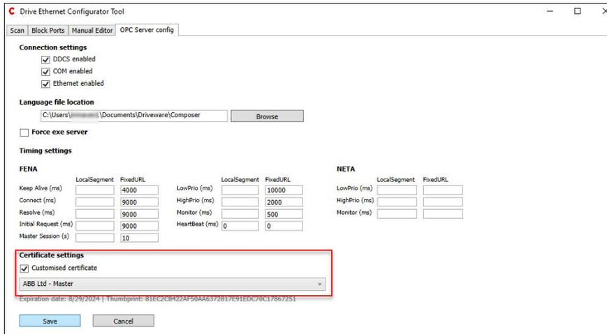
5. You will be prompted to restart the drive. Click **OK** to proceed. If certificate is validated, the drive successfully connects through HTTPS mode and indicates “🔒 Secure connection with custom certificate”.
