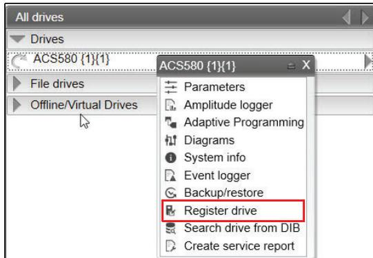
If you used the drive context menu, make sure that Drive Composer is connected online with the drive for successfully registering the drive. If you used **Tools** → **Register drive**, you can register the drive when Drive Composer is either in online/offline mode with the drive.
