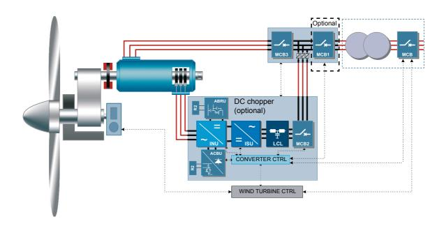
With the crowbar and the DC chopper, the wind turbine is capable of handling fault situations like rotor overspeed, short interruptions, voltage dips/sags and swells. With these energy absorbers, the converter is capable of meeting even the most strictest grid fault ride-through requirements in accordance with international grid codes.
