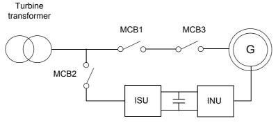
MCB1 stator breaker MCB2 converter contactor
