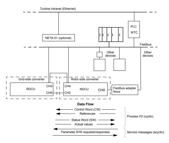
The converter can be set to receive all of its control information through the fieldbus interface, or the control can be distributed between the fieldbus interface and other available sources, eg, digital and analog inputs.
