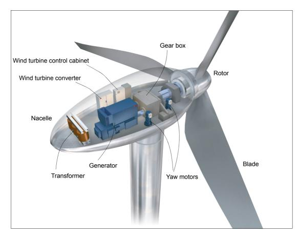
The main components of a wind turbine system are presented in the picture below.
