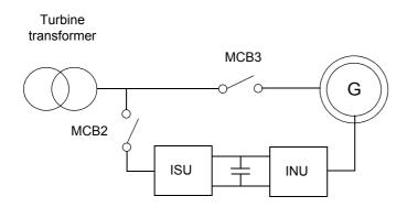
MCB2 converter contactor MCB3 stator breaker
