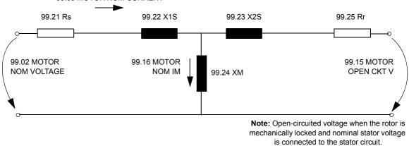
Since the application measures both rotor- and stator-side quantities, the identification run method is not used with doubly-fed induction generator control. The control needs to be given the following data (from the generator data sheet) manually.
