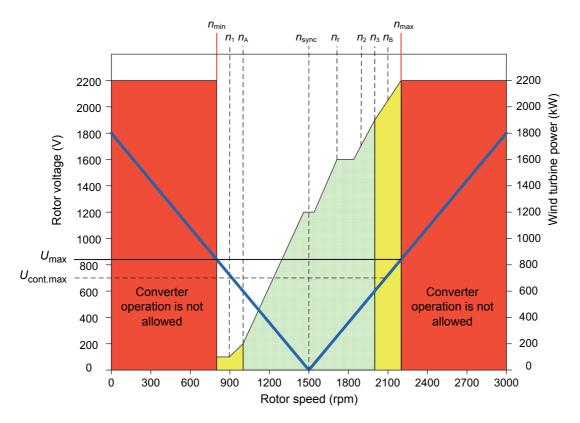
In operating range  $n_1...n_3$  the rotational speed is under normal operating conditions.
