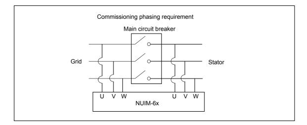
The following checks are automatically executed at start-up in the order in which they are listed:
