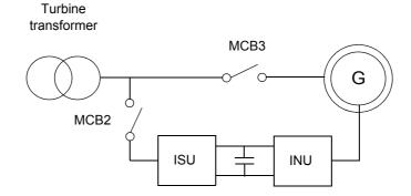
A typical procedure required to connect the wind generator to the grid is as follows:
