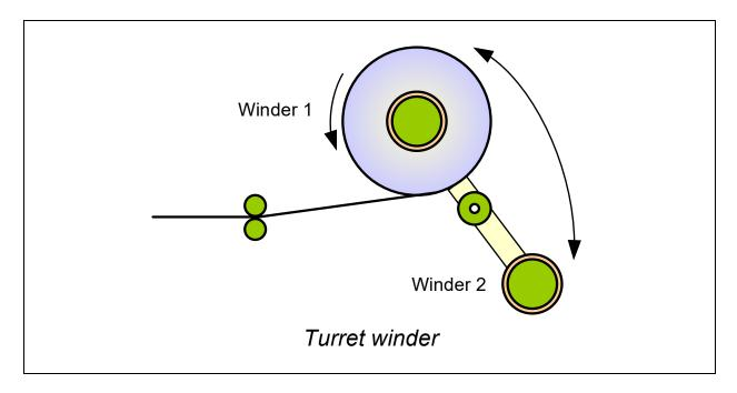
During the roll change, the web material is cut with a flying knife. To facilitate slicing of the material, torque boost defined by the user can be applied to temporarily increase the tension of the web. When the material is cut, the load cell or dancer is disconnected from the web and cannot therefore be used for the tension control. To finish the roll after cutting, the torque memorized before cutting can be used as the torque reference for the motor.
