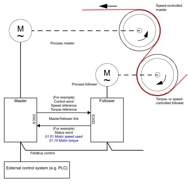
The master drive is typically speed-controlled and the other drives follow its torque or speed reference. In general, a follower should be
