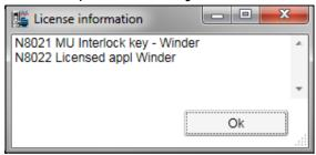
If the program was loaded to a ZMU-02 memory unit without the license key, then the drive indicates a fault *64A5 Licensing fault*. See the auxiliary fault code in the Event logger to know the plus code of the missing license, in this case N8021. For further assistance, contact your local ABB representative.
