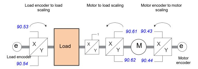
Any gear ratio between the load encoder and the load is defined by 90.53 Load gear numerator and 90.54 Load gear denominator. Similarly, any gear ratio between the motor encoder and the motor is defined by 90.43 Motor gear numerator and 90.44 Motor gear denominator. In case the internal estimated position is chosen as load feedback, the gear ratio between the motor and load can be defined by 90.61 Gear numerator and 90.62 Gear denominator.
