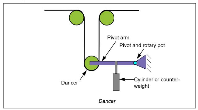
An advantage of a dancer is the web storage, which acts like an accumulator to absorb and isolate tension disturbances.
