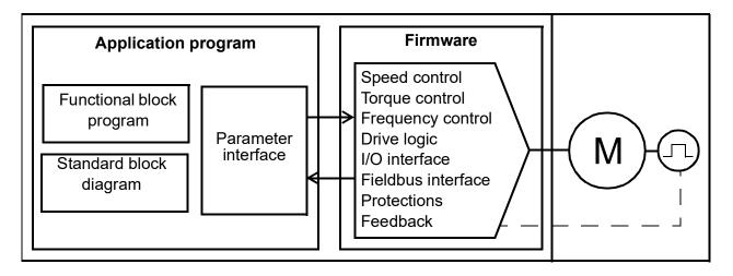
The firmware program performs the main control functions, including speed and torque control, drive logic (start/stop), I/O, feedback, communication and protection functions. Firmware functions are configured and programmed with parameters, and can be extended by application programming.
