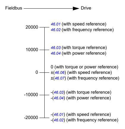
The scaled references are shown by parameters 03.09 EFB reference 1 and 03.10 EFB reference 2.
