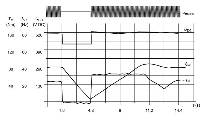
$U_{\mathrm{DC}}$ = intermediate circuit voltage of the drive,  $f_{\mathrm{out}}$  = output frequency of the drive,  $T_{\mathrm{M}}$  = motor torque Loss of supply voltage at nominal load ( $f_{out}$  = 40 Hz). The intermediate circuit DC voltage drops to the minimum limit. The controller keeps the voltage steady as long as the mains is switched off. The drive runs the motor in generator mode. The motor speed falls but the drive is operational as long as the motor has enough kinetic energy.
