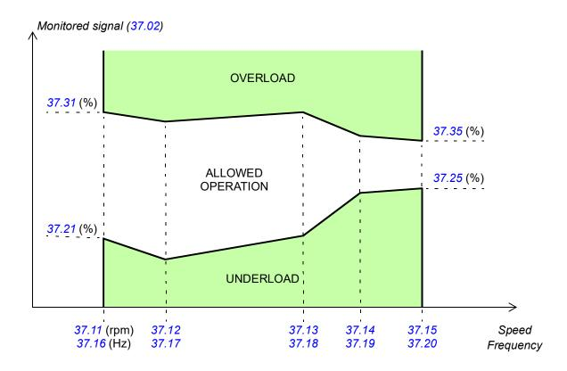
The action (none, warning or fault) taken when the signal exits the allowed operation area can be selected separately for overload and underload conditions (parameters 31.03 and 31.04 respectively). Each condition also has an optional timer to delay the selected action (37.41 and 31.42).
