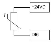
The resistance of the PTC sensor increases when its temperature rises. The increasing resistance of the sensor decreases the voltage at the input, and eventually its state switches from 1 to 0, indicating overtemperature.
