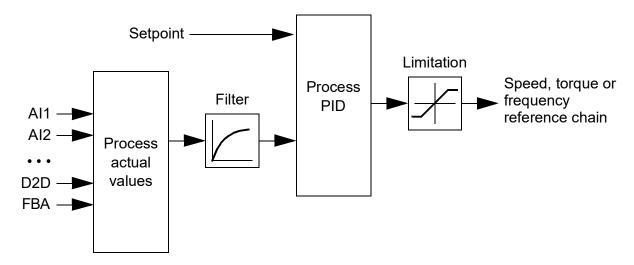
The control program contains two complete sets of process PID controller settings that can be alternated whenever necessary; see parameter 40.57 PID set1/set2 selection.
