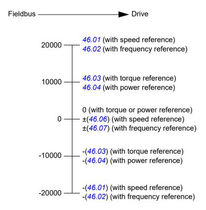
The scaled references are shown by parameters 03.05 FB A reference 1 and 03.06 FB A reference 2.
