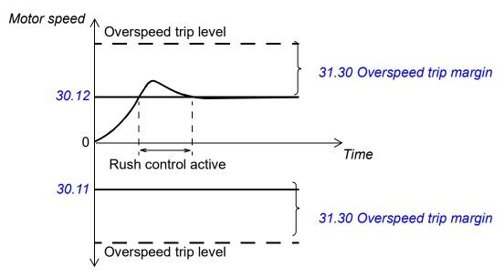
The function is based on a PID controller. The proportional gain and integration time can be defined by parameters. Setting these to zero disables rush control.
