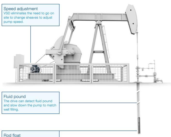
Movement can be slowed down and speeded up as the rod starts to fall through high viscosity oil.
