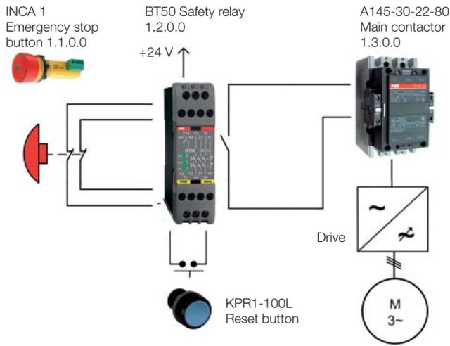
Figure 2: Connection example of the emergency stop function with a contactor.
