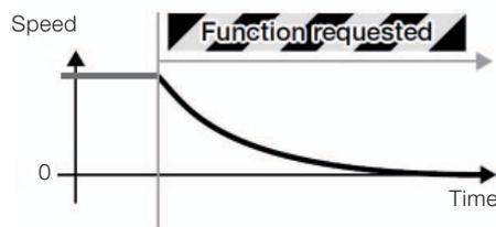
Figure 1: Typical motor speed with stop category 0 stop.
