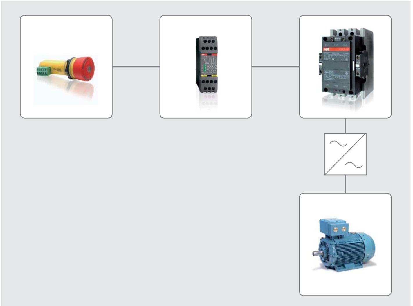
This document presents details how an emergency stop, stop category 0, safety function can be designed by using ABB drives together with safety devices and contactors. The safety function is implemented according to EN/IEC 62061, EN ISO 13849-1, EN ISO 13850, EN/IEC 60204-1 and EN/IEC 61800-5-2 machinery standards. Necessary SIL/PL calculations are presented using ABB's Functional safety design tool.
