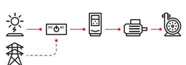
The ABB solar pump drive can also be equipped to operate from the grid if no solar power is available.
