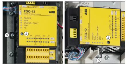
4. Make sure that the FSO data cable (terminal X110) is connected to the drive. Use only the cable delivered with the module.
