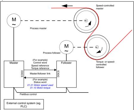
The master drive is typically speed-controlled and the other drives follow its torque or speed reference. In general, a follower should be
