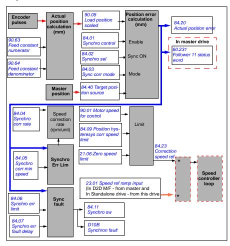
The first part of the synchro control function is the basic function described in *Synchro control function - block diagram* (page *90*). The second part of the synchro control function is the synchro correction with parameter *84.04 Synchro corr rate* in combination with different limit conditions. See description in parameter *84.05 Synchro corr min speed*.
