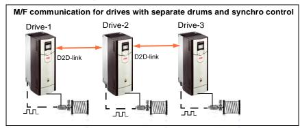
In a synchro control, the speed reference and position of the master drive are transmitted to the follower drives. The follower drives are in speed control mode with speed correction, where the position of the follower drives is compared with the position of the master drive and the required speed correction is added to its own speed reference chain. For more information, see Shaft synchro control (page 90).
