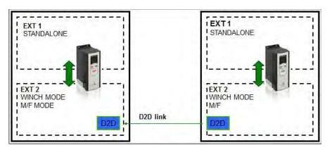
D2D-link: In each drive the M/F communication in the D2D-link is activated with parameter 60.200 Winch drive type by selecting the appropriate drive type.
