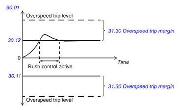
The function is based on a PI controller. The proportional gain and integration time can be defined by parameters. Settings these to zero disables rush control.
