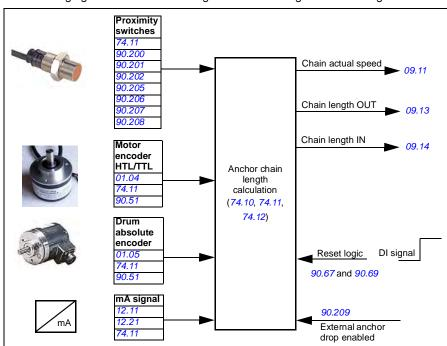
The following figure shows a block diagram of measuring the actual length of a chain.
