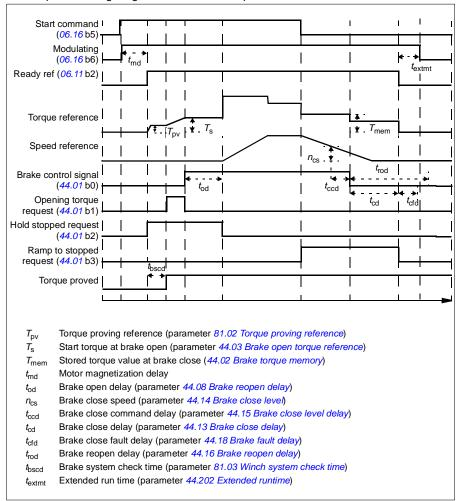
**Note:** In case of any fault, the brake will close immediately. The brake control uses relay output RO1 as default.
