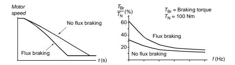
The drive monitors the motor status continuously, also during flux braking. Therefore, flux braking can be used both for stopping the motor and for changing the speed. The other benefits of flux braking are:
