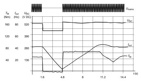
$U_{DC}$ = intermediate circuit voltage of the drive,  $f_{out}$  = output frequency of the drive,  $T_{M}$  = motor torque Loss of supply voltage at nominal load ( $f_{\text{out}} = 40 \text{ Hz}$ ). The intermediate circuit DC voltage drops to the minimum limit. The controller keeps the voltage steady as long as the mains is switched off. The drive runs the motor in generator mode. The motor speed falls but the drive is operational as long as the motor has enough kinetic energy.
