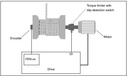
When parameter 78.04 Slip detection mode is set to Internal, slip detection is based on the comparison of drive speed, drive torque and chain speed (measured by an encoder) with the supervision limits. The new reference (protection speed) is applied after a predefined delay (parameter 78.09 Activation delay time).
