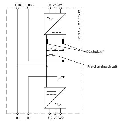
Each drive has an independent DC capacitor pre-charging circuit.
