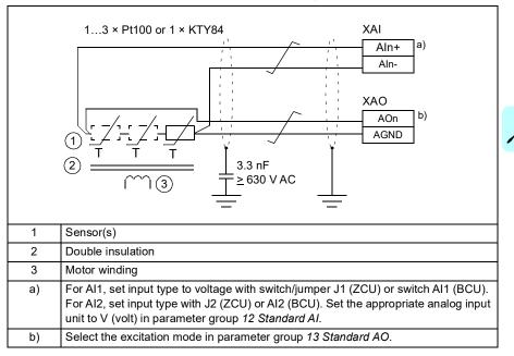
For the connection alternatives, refer to *Implementing a motor temperature sensor connection* on page 68.
