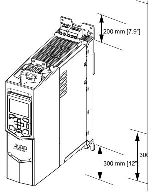
**Note**: The temperature of the cooling air entering the unit must not exceed the maximum allowed ambient temperature (see *Ambient conditions* on page 132). Consider this when installing heat-generating components (such as other drives, mains chokes and brake resistors) nearby.
