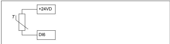
One PTC sensor can be connected to digital input DI6.
