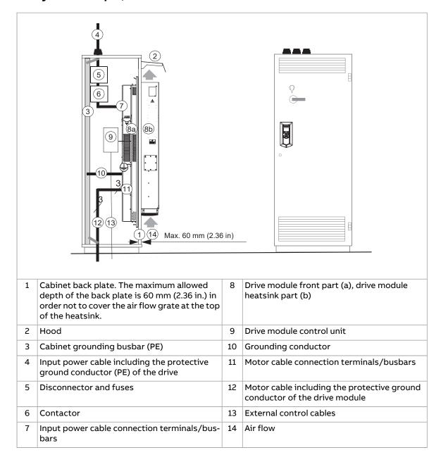
**Note:** The power cable shields can also be grounded to the drive module grounding terminals.
