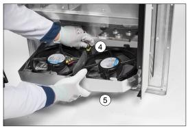
To replace the main cooling fans from the back side:
