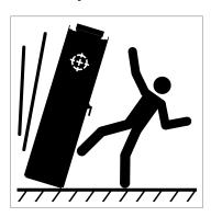
Be careful when handling a tall module. The module overturns easily because it is heavy and has a high center of gravity. Whenever possible, secure the module with chains. Do not leave an unsupported module unattended especially on a sloping floor.
