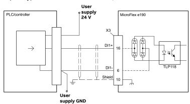
Digital input - typical connections from a PLC/controller:
