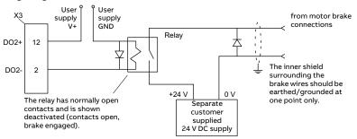
This circuit uses DO2 as a motor brake output. The output is configured using Mint keyword MOTORBRAKEOUTPUT; see the Mint help file for details. With this configuration, the following sequences can be used to control the brake. To engage the brake:
