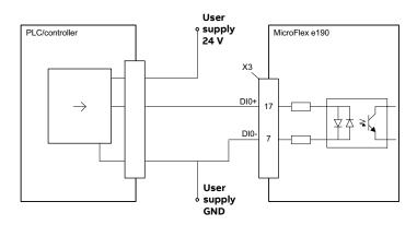
Digital input - typical connections from an ABB DO561 PLC output module:
