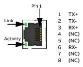
The E1 and E2 Ethernet ports on the top panel of the MicroFlex e190 are used for real-time Ethernet fieldbus connections such as EtherCAT®, Ethernet POWERLINK® and PROFINET®. For full details about the fieldbus connections, see the Mint Workbench help file.
