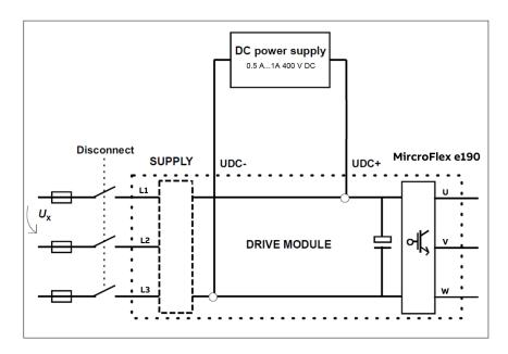
Note: Limit the reforming current to max. 200 mA. If the DC power supply does not have an adjustable current limiter, increase the voltage gradually from 0 V to 400 V.
