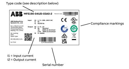
The first digit of the serial number refers to the manufacturing plant. The 2nd and 3rd digits indicate the year of manufacture, while the 4th and 5th digits indicate the week. The 6th digit indicates the rating. Digits 7 to 10 are a running integer starting every week at 0001.
