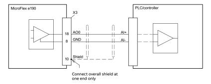
Analog output - typical connections to an ABB AI523:
