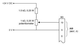
Analog input - typical connections from a PLC/controller:
