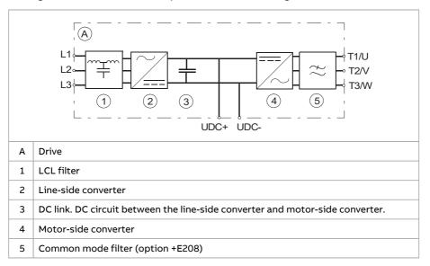
The line-side converter rectifies three phase AC current to direct current for the intermediate DC link of the drive. The intermediate DC link further supplies the motor-side converter that runs the motor.
