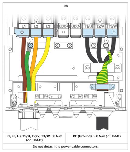
For frame R8: Install the side plates if removed.
