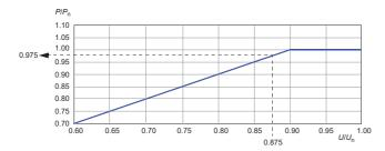
Example 1:  $P_n$  for ACS880-11-045A-3 is 22 kW. The supply voltage (U) is 350 V.
