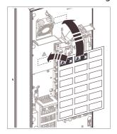
3. For frames R6 and R8: Remove the shroud on the power cable terminals.
