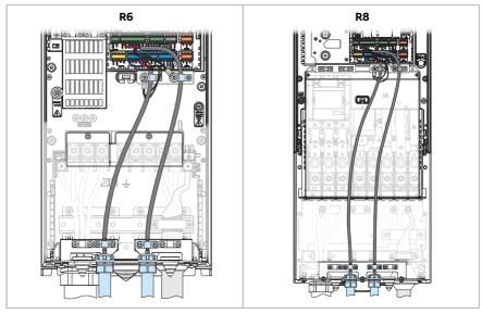
9. Connect the conductors to the appropriate terminals of the control unit and tighten to 0.5 ... 0.6 N·m (0.4 lbf·ft).
