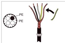
Only allowed for input cabling with phase conductor cross-section less than 10 mm<sup>2</sup> (8 AWG)
