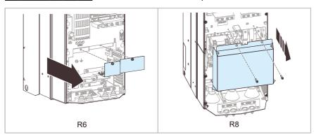
4. For frame R6: If you need more working space, unscrew the screw and lift the EMC plate off. Install the EMC plate again after you have installed the motor and input power cables.
