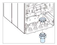
8. Cut the cables to suitable length (note the extra length of the grounding conductors). If you use a symmetrically shielded VFD cable, twist the grounding wires together with the cable shield and connect them to the grounding terminals. Ground the shield 360° at the clamp. If you use discrete conductors connect the insulated ground conductor to the grounding terminal.
