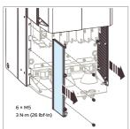
6. Remove the rubber grommets of the cables to be installed from the cable entry plate. Install the grommets downwards in unused holes.
