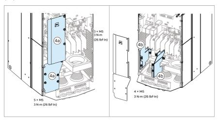
5. For frame R8: For easier installation, you can remove the side plates.
