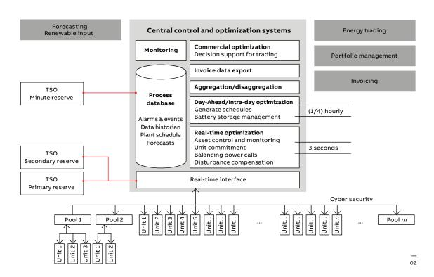
ABB Ability Virtual Power Pools is a control and optimization system to automate control of power generation units, storages and controllable loads.
