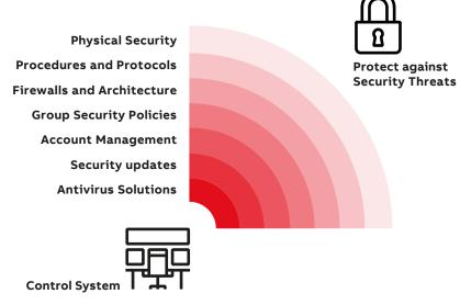
ABB recommends a defense in depth approach with multiple layers of protection placed throughout the system to shield systems and data from threats. Current and validated security updates on site are a key factor to reach the next level of cyber security. The Security Update Service distributes updates in a secure, automated and controlled way to customer sites.
