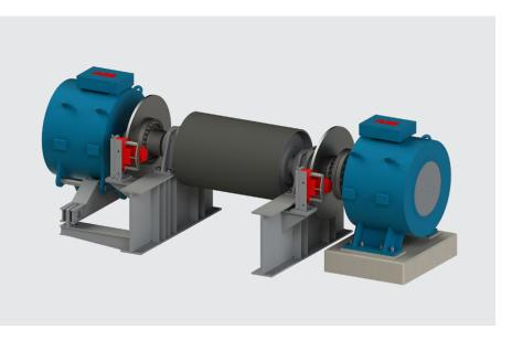
ABB's gearless conveyor drive, rated from 1 to 3 MW motor power, removes the need for a gearbox, thereby lowering maintenance costs while improving overall reliability leading to greater uptime.
