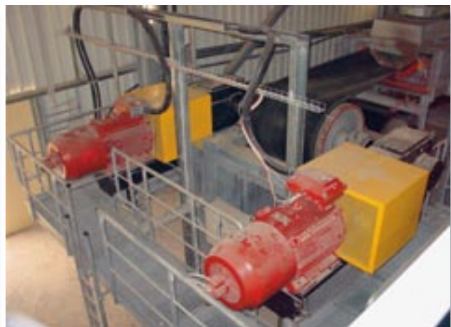
Figure 9: Configuration of the troughed belt conveyor tail end and drives
