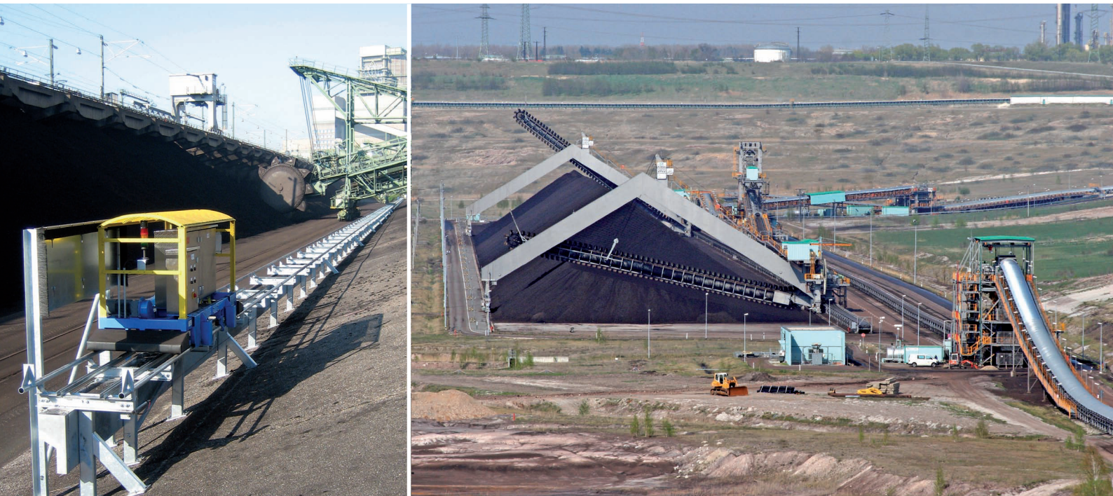
Fig. 1: 3D scanners deliver information for stockpile monitoring and visualisation in an integrated coal management system.
