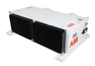
The BORDLINE® M30 DC static converter is a compact, rugged unit used to generate onboard supply voltages for light rail vehicles. Due to its wide input voltage range, the converter works with nominal grid voltages of 600 Vdc and 750 Vdc. The integrated input filter allows the converter to be connected directly to the catenary line.
