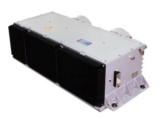
The BORDLINE® M35 DC static converter is a compact, rugged unit used to generate onboard supply voltages for light rail vehicles. Due to its wide input voltage range, the converter works with nominal grid voltages of 600 Vdc and 750 Vdc. The integrated input filter allows the converter to be conncted directly to the catenary line.
