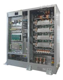
The Compact Converter BORDLINE® CC1500 AC converts the power from 15 kV/16.7 Hz or 25 kV/50 Hz line into propulsion power for the traction motors and auxiliary power for onboard consumers.
