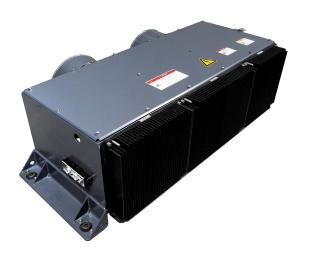
The BORDLINE® M25 AC 1000 static converter is a compact, rugged unit used to generate onboard three-phase AC voltage for passenger coaches. This unit is part of ABB's BORDLINE® M product platform for onboard converters. The converter can be connected directly to the 1000 Vac/16.7 Hz train line.
