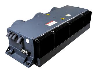
The BORDLINE® M45 AC static converter is a compact, rugged unit used to generate onboard supply voltages for passenger coaches from the train line. This unit is part of ABB's BORDLINE® M product platform for onboard converters. The converter can be connected directly to the 1000 Vac/16.7 Hz train line.
