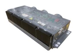
The BORDLINE® M50 AC static converter is a compact, rugged unit used to generate onboard supply voltages for passenger coaches from the train line. This product is part of the ABB BORDLINE® M platform for onboard converters. The converter can be connected directly to the 1000 Vac/16.7 Hz train line.
