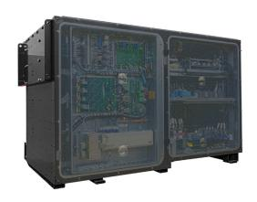
BORDLINE® CC750 MS converts the power from the 15 kV/16.7 Hz or 25 kV/50 Hz line into propulsion power for the traction motors and auxiliary power for onboard consumers (AC, DC and battery). Alternatively, the Compact Converter can be fed with a diesel genset for the non-electrified 'last mile'.
