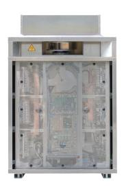
The BORDLINE® M80 AC static converter is a compact, rugged unit used to generate onboard supply voltages for passenger coaches from the train line. This product is part of the ABB BORDLINE® M platform for onboard converters. The converter can be connected directly to the 1000 Vac/16.7 Hz train line.
