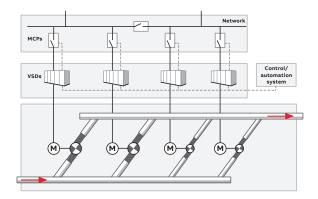
Operating parallel pumps with variable speed drives.
