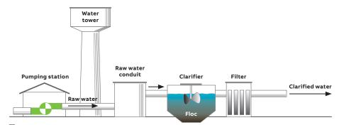
Solid contact sedimentation water treatment process.
