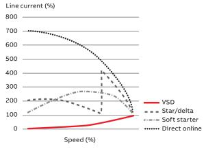
This results in less stress on motors, pumps and mechanical parts, a reduction of maintenance costs and a longer lifetime of the equipment.
