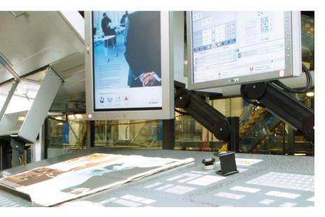
The soft-proof viewer, an extension to the MPS Control Console, provides the printer with a color image of the pages of the product currently being printed. The image displayed is selected automatically by the control console without any additional input from the printer being necessary – whichever page is currently selected on the console is displayed as a soft-proof.
