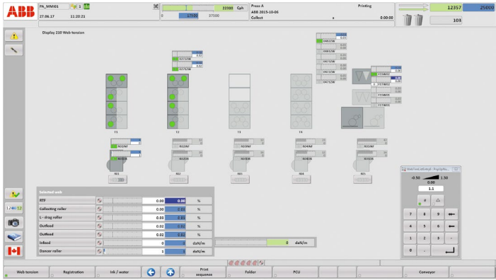
Fig. 4: Web tension display with numerical keypad for the entry of a new reference value
