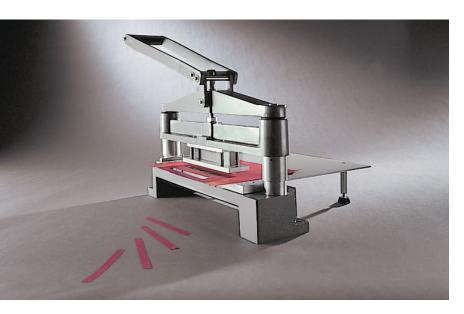
L&W Strip Punch provides you with precisely cut sample strips, which can be used in tensile strength tests, fracture toughness tests, compression strength tests, bending stiffness tests, or ring crush tests.
