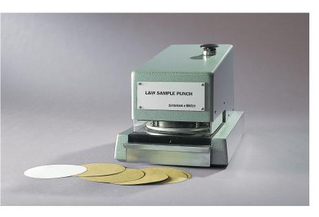
L&W Sample Punch is intended for easy and rapid preparation of circular test pieces to be used in the determination of grammage. The punch is pneumatically operated forease of use and the specially designed sample holder ensures extremely good cutting results on both thin and tough materials.
