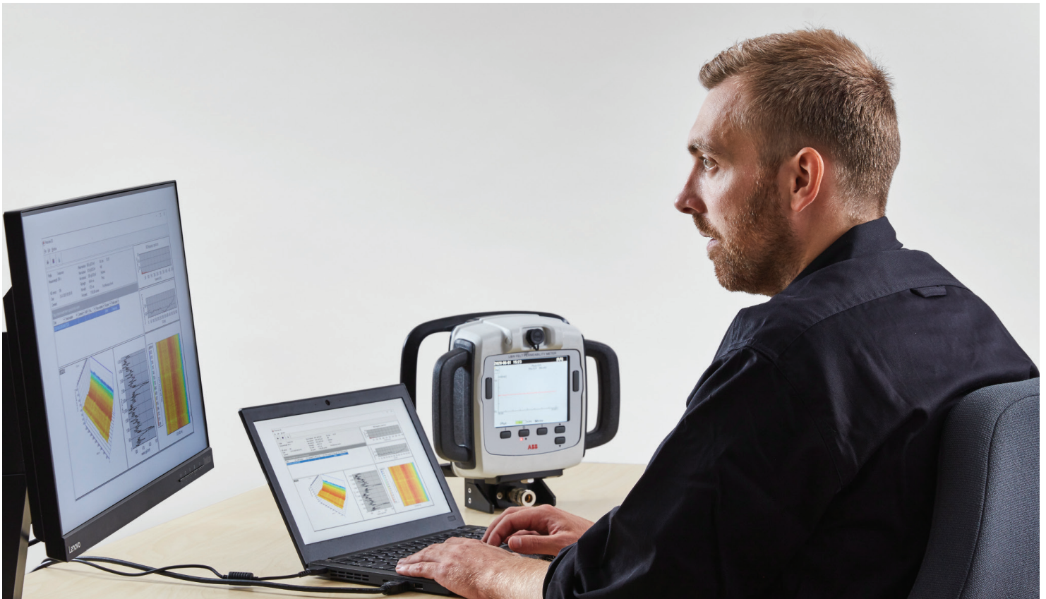
03 The L&W PressView 3D PC software has a database for trends and advanced analysis (CD/MD, 2D+3D, FFT, etc.).
