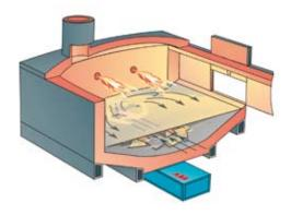
In metallurgical processing, effective and reliable stirring of the melt is one of the prerequisites for higher productivity and improved process performance. In over 1200 installations, the steel and aluminium industry have chosen non-contact electromagnetic stirring technology, invented and continuously adapted by ABB, to deliver necessary long-term and important viable results.
