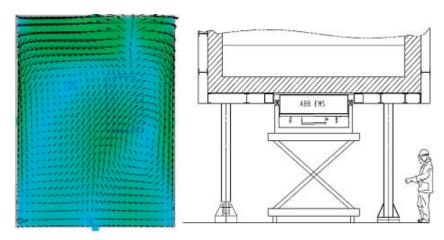
Simulation tools are based on 1200 EMS installations and quickly indicate a possible solution, project payback and performance guarantee for any 5-200 tonne furnace. At AMAG Rolling the result is effective stirring of the entire melt, ~1 rotation/minute.
