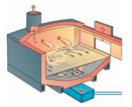
In metallurgical processing, effective and reliable stirring of the melt is one of the prerequisites for higher productivity and improved process performance. In over 1200 installations, the steel and aluminium industry has chosen non-contact electromagnetic stirring technology, invented and continuously adapted by ABB, to deliver necessary long-term and important viable results.
