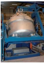
Left picture: Simulation tools are based on 1200 EMS installations and quickly indicate a possible solution, project payback and performance guarantee. At Ljunghäll AB the result is effective stirring of the entire melt, ~1 rotation/minute.
