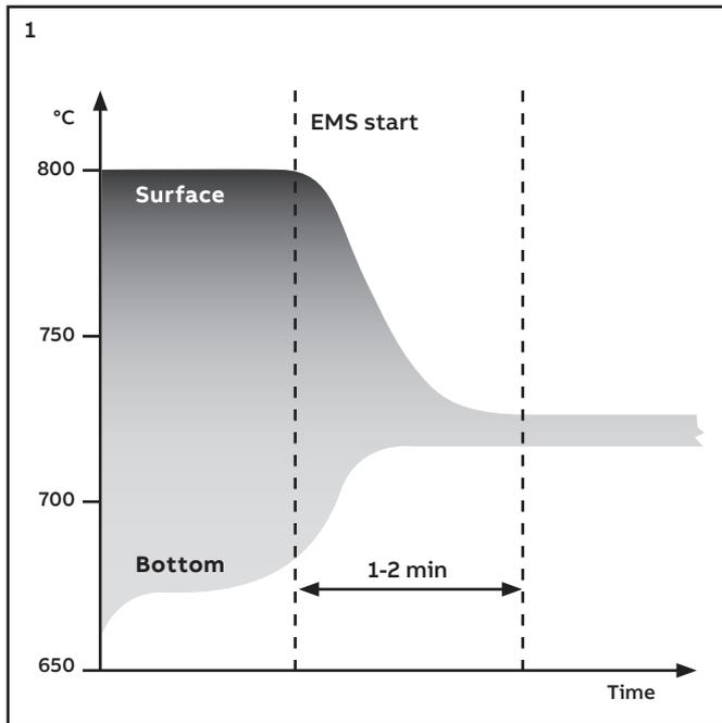
1 Schematic sketch of the temperature homogenization when AL-EMS is turned on
