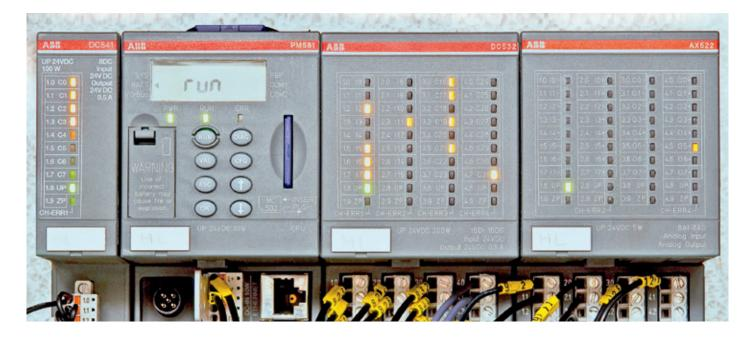
The Global Underground Mining Service Center of ABB in Sweden has worldwide responsibility for mine hoist systems and has developed an upgrade kit to replace the old analogue brake card BCC for ABB's mine hoist brake systems. This upgrade kit comprises the new digital technology used by ABB.
