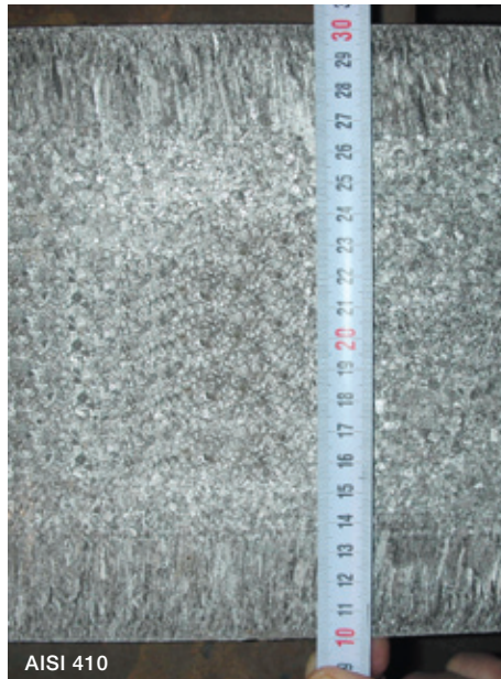
Structures achieved with the new ABB stirrers for AISI 410.
