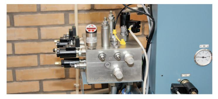
The Global Underground Mining Service Center of ABB in Sweden has worldwide responsibility for mine hoist systems and has developed an upgrade kit for the Bosch Rexroth hydraulic unit for ABB's mine hoist brake systems. The upgrade kit comprises a new valve block that includes the latest valves and technology used by ABB.
