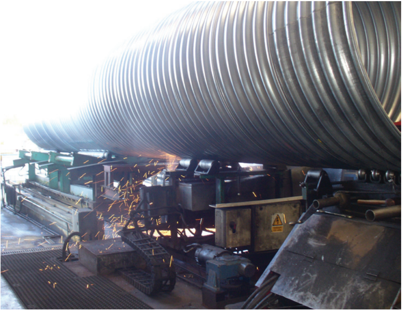
A rotating and forward-moving pipe run being cut into sections. The saw moves with the pipe to create a perfect, right-angled cut.
