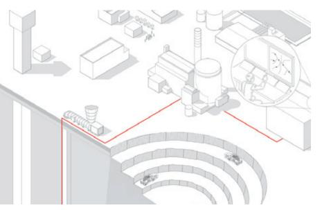
ABB's SmartVentilation is a complete mine ventilation control solution with ventilation on demand functionality. It is a modular system which can be fully integrated into ABB's 800xA control system. Efficient use of your ventilation system and improved air quality by providing fresh air where necessary will result in energy savings of up to 30-50 % per year.
