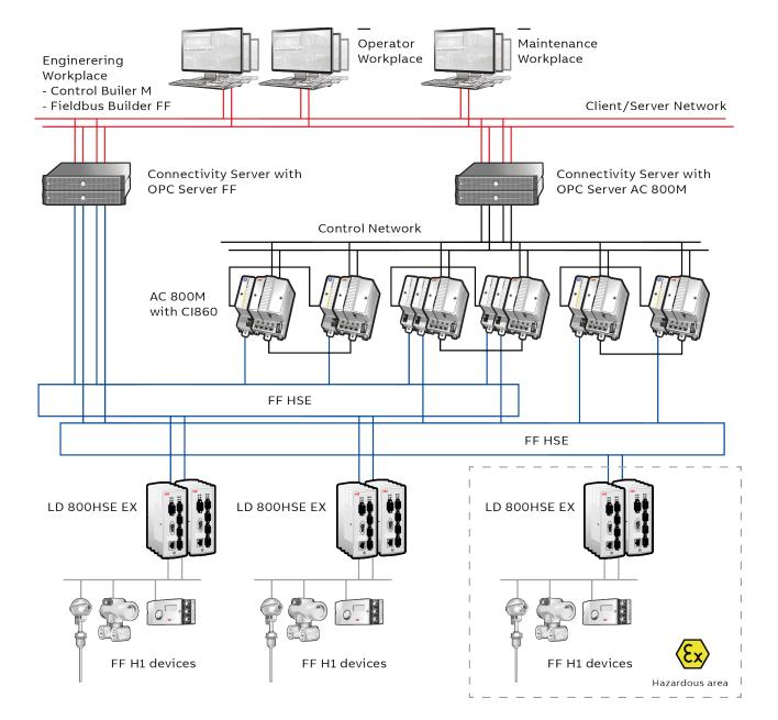
Figure 1. Sample System Structure with FF Network
