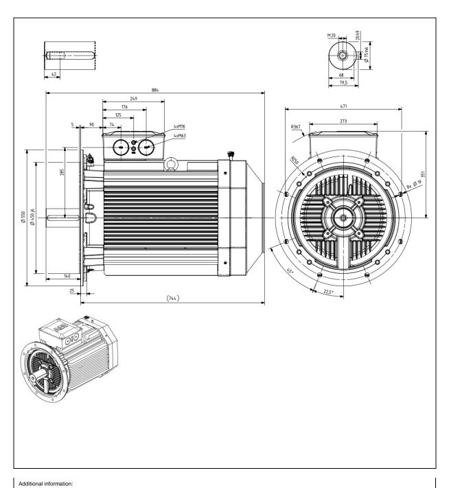
Ex ec / Ex t Motor Type: Document No: M3AA 280 (G, K) 4-8p B5 **Dimension Print** 3GZL500828-3 Description: Three phase motor ABB Oy, Motors and Generators M. Szymanski Unit: Issued by: Replaces: 2017-03-24 J. Cieslikowski Date: Approved by: Replaced by: Customer Reference: <u>ABB</u> **ABB** Oy
